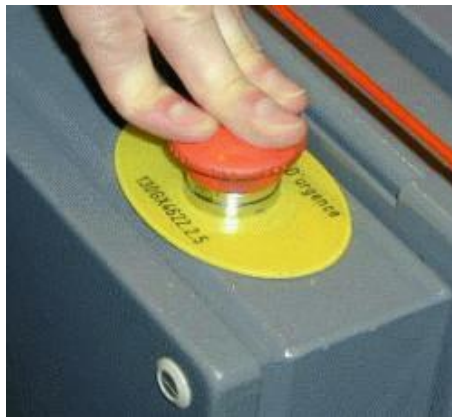
Figure 16. The emergency stop pushbutton
